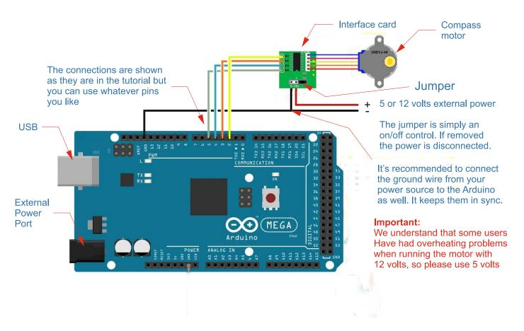
This diagram shows a full size Arduino Mega Card, but there is also a smaller Mini Mega which is quite a bit cheaper. It has the same number of pins and because of it's size is easier to mount inside the cockpit structure. However many people prefer the larger card which can be easier to work with.
